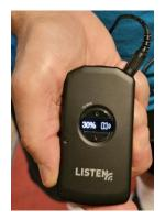
Whether you are using the hearing aid loop or the earpiece, you can adjust the volume using the UP/DOWN buttons on the front of the receiver.
